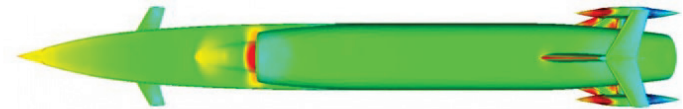
Figure 5. BLOODHOUND SSC config10 top – note the long and slender shape to minimise air compression and hence drag.
