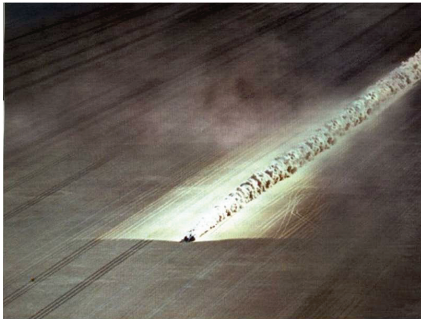
Figure 4 – The supersonic shock wave emanating from the nose of ThrustSSC and showing up late in the afternoon intensified by a dust storm earlier in the day.
